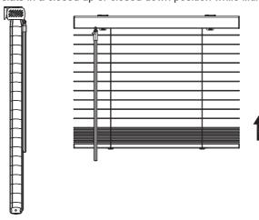
▲ To avoid offset stacking (bottom rail not hanging straight downward), hold the bottom rail with both hands evenly, and lift/pull while keeping the underside of the bottom rail pointed straight down.
