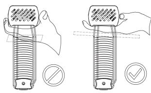
Push the headrail in towards the brackets to activate the spring-loaded tab and in the same motion tilt the back of the headrail downwards at the angle. Make sure your blind is secure.
