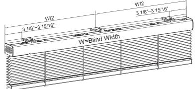
Brackets should not interfere with the tilt mechanism.
