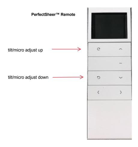
PerfectSheer<sup>™</sup> has a dedicated remote control to take full advantage of the shade's capabilities. While it looks similar to the remote used to control all of our other motorized shades, the PerfectSheer<sup>™</sup> remote has 2 additional features to the left of the up/down buttons. When pressed, the buttons allow you to tilt the shade's vanes up and down. The buttons can also be used to micro adjust the vane position when setting limits during programming.
