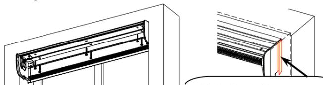
Light block film to cover the light between wall and housing end cap.
