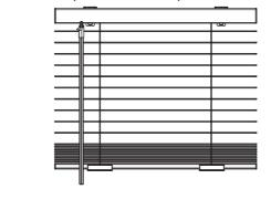
A To avoid offset stacking (bottom rail not hanging straight downward), hold the bottom rail with both hands evenly, and lift/pull while keeping the underside of the bottom rail pointed straight down.
