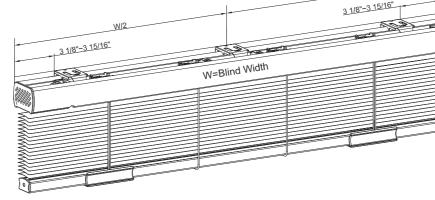
A Brackets should not interfere with the tilt mechanism.
